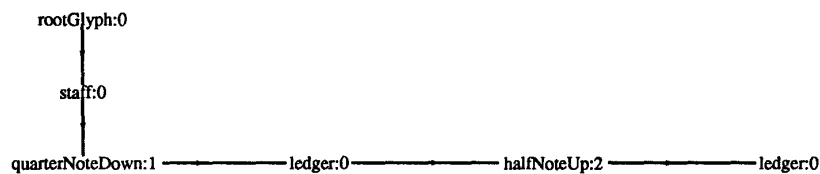
Figure 5.11: LedgerLines. Note that _ledgerlines always display 6 lines. As the corresponding TTree shows, _ledgerLines exist at the same hierarchical level as the notes they are associated with.
