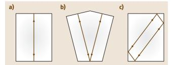
Fig. 9.32 Room shapes causing risk of flutter echoes
