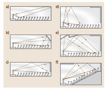
Fig. 9.34 Means of controlling early reflections in auditoria (after [9.28])
