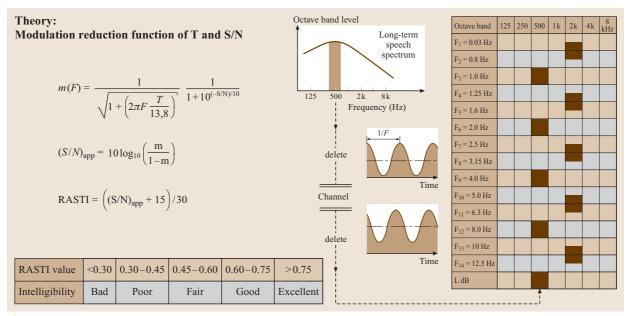
Fig. 9.10 Illustration of the theory and principle in the measurement of STI or RASTI. The scale for the evaluation of RASTI values is shown at the bottom (after [9.13])
