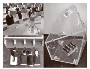
Fig. 9.16 Model audience used in a 1:10 scale model of the Danish Broadcasting concert hall shown in Fig. 9.15. Upper-left corner: Close view of model orchestra musicians and spark sound source. Lower left: close-up view of model chairs and polystyrene audience with hollow chest. Dress and hair is made from wool felt. Right: model audience and chairs placed in model reverberation chamber for absorption testing (reverberation room designed by Nagata Acoustics)
