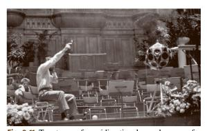
**Fig. 9.11** Two types of omnidirectional sound sources for room acoustic measurements: blank pistol (in the *raised hand of the seated person*) and an omnidirectional loudspeaker (icosahedron with 20 units)
