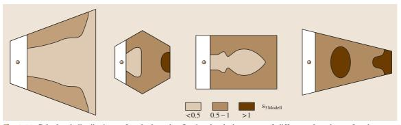
Fig. 9.20 Calculated distributions of early lateral reflection levels in rooms of different plan shape: fan, hexagon, rectangular and reverse fan. Darker areas represent higher LEF levels (after [9.5])
