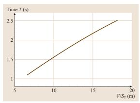
Fig. 9.28 Reverberation time T in occupied concert halls versus the ratio between the volume V and area occupied by the audience and orchestra  $S_{\rm T}$  (including aisle space up to 1 m width). Derived from empirical data (after [9.9])
