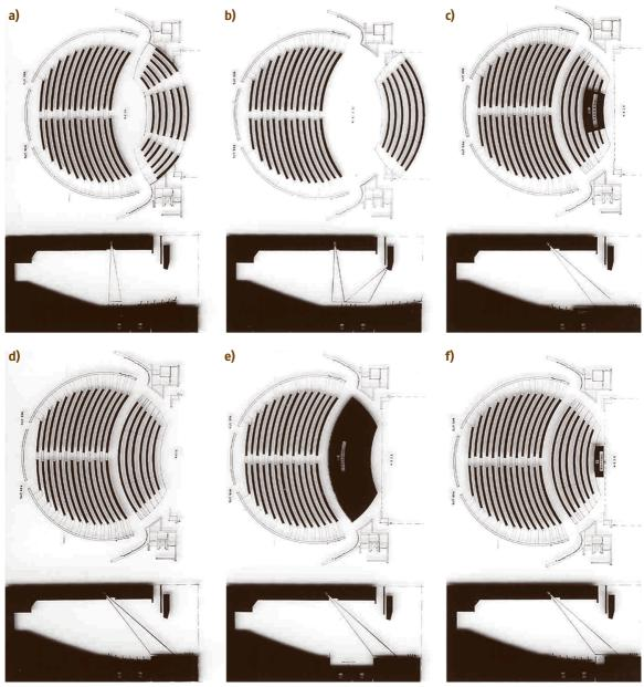
Fig. 9.43a-f Plans showing a flexible theater in Hëlsingborg, Sweden, with different layouts of the stage, orchestra pit and audience seating. (a) and (b): arena with small and large stage respectively, (c), (e), and (f): proscenium theater with three different sizes of orchestra pits. (d): proscenium theater without pit
