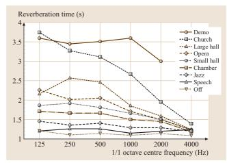
Fig. 9.57 Reverberation time values measured in a hall for different settings of the reverberation enhancement system (LARES)
