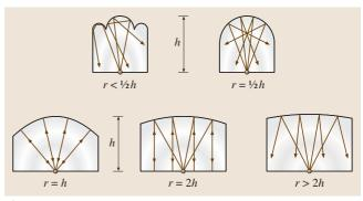
Fig. 9.30 Focusing by concave ceilings (after [9.31])
