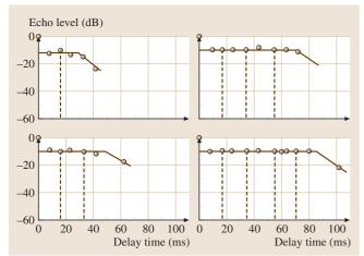
**Fig. 9.4** Thresholds of perception of a new reflection (*circles* and *horizontal lines*) being added to impulse responses already containing one, two, three, or four other reflections with delay and relative levels, as indicated by the *vertical lines* (after [9.5])
