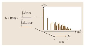
Fig. 9.7 The definition of strength G: the total energy in the impulse response measured relative to the direct sound level at 10 m distance from the source
