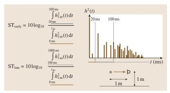
Fig. 9.9 The definition of early support ST<sub>early</sub> and late support ST<sub>late</sub>, the ratio between early and late reflection energy respectively and the direct sound in the impulse response. Both are measured at 1 m distance from the source
