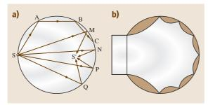
Fig. 9.31a,b Circular room with focused and creeping waves (a), and with the surface shape modified (b) so that these phenomena are avoided
