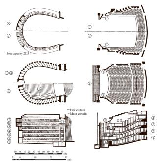
Fig. 9.44 Plan and section drawings of the Teatro alla Scala, Milan, Italy, from 1778 (left) and the New National Theatre Opera, Tokyo, Japan, from 1997 (*right*) (after [9.3])
