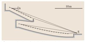
Fig. 9.24 Section of a hall with a rear balcony and constant clearance. The result is an increased slope for the elevated balcony (after [9.30])
