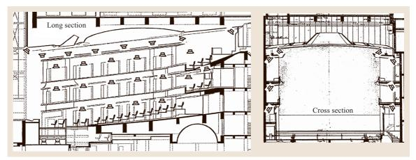
Fig. 9.56 Example of distribution of loudspeakers for reverberation enhancement in a theatre
