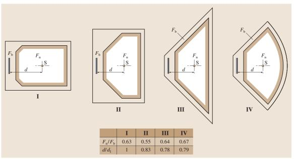
Fig. 9.19 Mean stage-listener distance and net efficiency of floor area for four different room shapes.  $F_n$  is the net area occupied by the audience,  $F_b$  is the total floor area, d is the average source-listener distance;  $d_I = d$  for case I (after [9.28])
