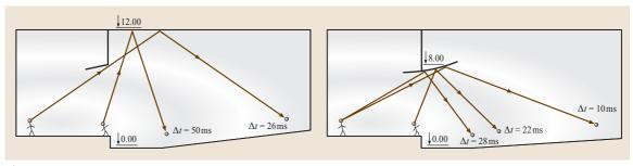
Fig. 9.38 The influence on reflection paths of a reflecting panel suspended in front of a stage (after [9.33])
