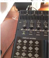
One thing to remember: The red peak signal is not on at all time no matter what you are doing. If you are using condensed microphone, remember to turn on +48V.
