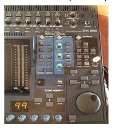
By doing this, you are connecting your microphone, to the 1st channel, to the 1st layer speaker, which you can then control using the mixer.
