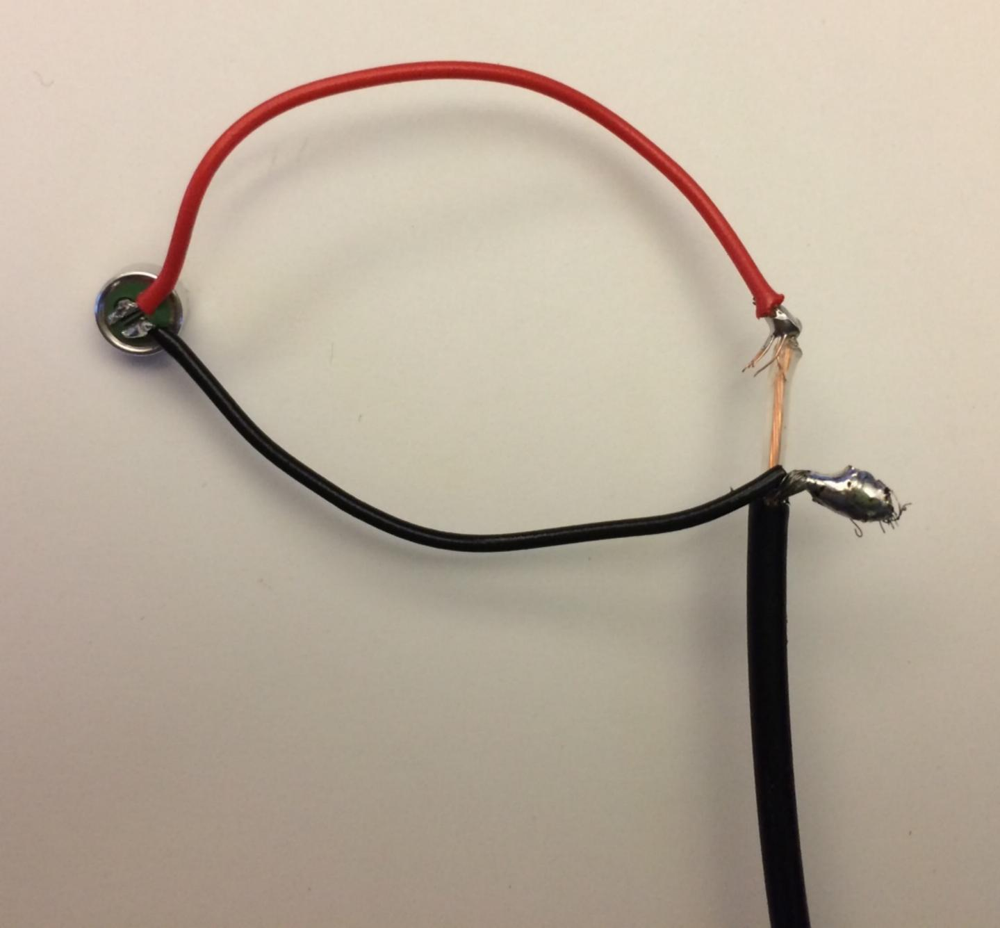
When you are done with all of these steps, carefully use electrical tape to wrap the individual connections, making sure to not allow any short circuits.
