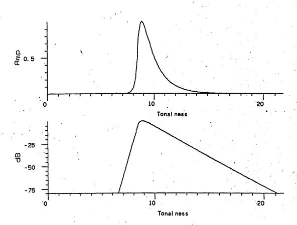
FIGURE 1: Computer simulations of masking patterns, modeled after Ziwcker [1955]. The model consists of exponential skirts with a 3rd-order polynomial joining the two exponentials. These curves are centered around 9 Bark. The high-frequency skirt has a fall-off rate 7 times that of the low-frequency side. The polynomial matches the slopes as well as the values at the joints.
