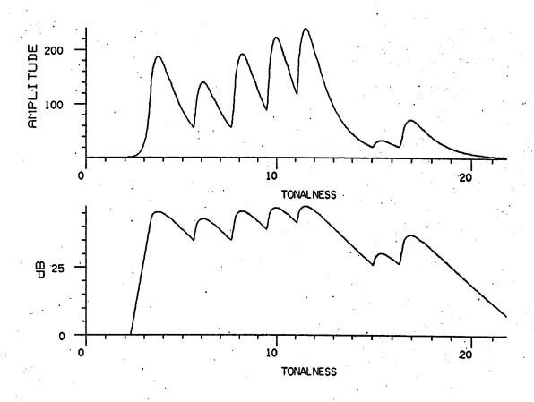
FIGURE 3: Simulated masking pattern based on the analysis of an oboe tone. The oboe tone has many harmonics of almost equal amplitude, unlike the clarinet which represents largely odd harmonics.
