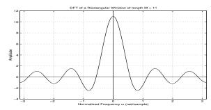
This (real) result is for the *zero-centered* rectangular window. For the *causal* case, a linear phase term appears:
