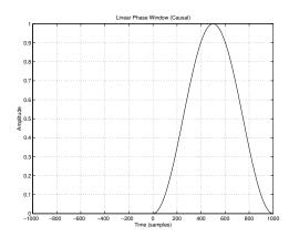
By shifting the original window in time by half its length, we have turned the original non-causal window into a causal window. The Shift property of the Fourier Transform tells us that we have introduced a linear phase term.
