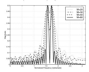
The preceding figures suggest that, for a rectangular window of length  ${\cal M}$ , two sinusoids can be most reliably
