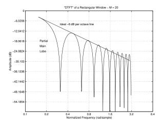
As the sampling rate approaches infinity, the rectangular-window transform (asinc) converges exactly to the sinc function. Therefore, the departure of the roll-off from that of the sinc function can be ascribed to aliasing in the frequency domain, due to sampling in the time domain.
