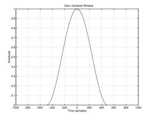
This may be called a "zero-centered" (or "zero phase", or "even") window function, which means its phase in the frequency domain is either zero or  $\pi$ , as we will see in detail later. (Recall that a real and even function has a real and even Fourier transform.) The window is also nonnegative, as is typical.
