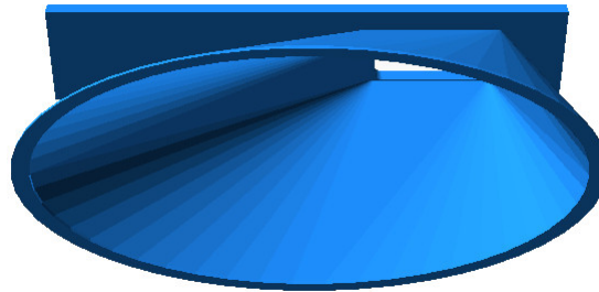
Figure 4.1: CAD Model of a Generic Passive Amplifier for the Built-In Speakers of a Mobile Device.
