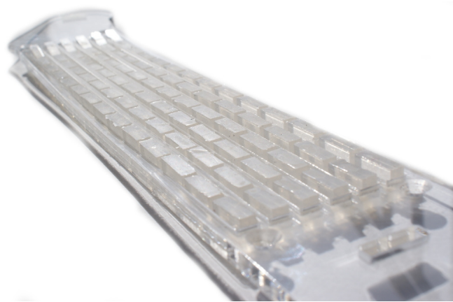
Figure 2.12: BLADEAXE1 Neck Based on Silicon Buttons.
