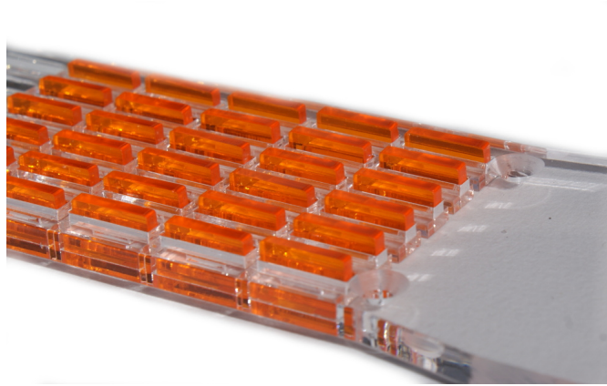
Figure 2.13: First Version of the BLADEAXE1 Laser Cut Acrylic Buttons.
