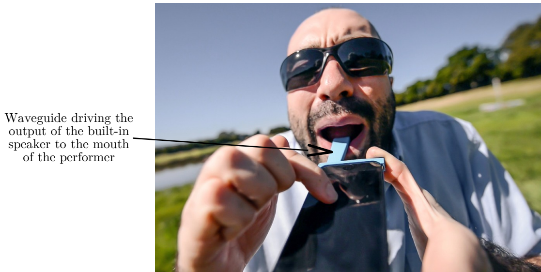
Figure 4.7: Mouth Resonator for Mobile Device Built-In Speaker.
