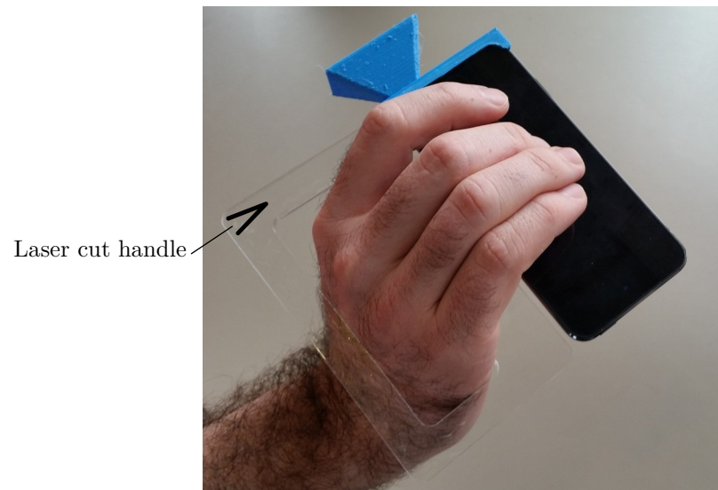
Figure 4.11: Single-Hand-Held Musical Instrument Based Using a Laser-Cut Plastic Handle.
