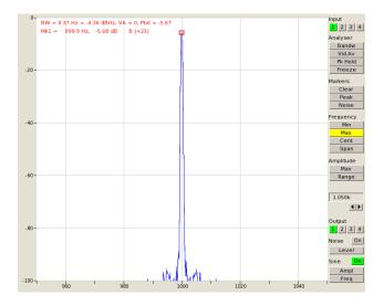
The next figure shows the effect of recovered audio clock jitter due to received packet timing differences when we add another instance of jack-mamba sending silence to the Mamba box (no other changes). This is using jaaa peak hold and averaging functions to see the worst long term distortion products:
