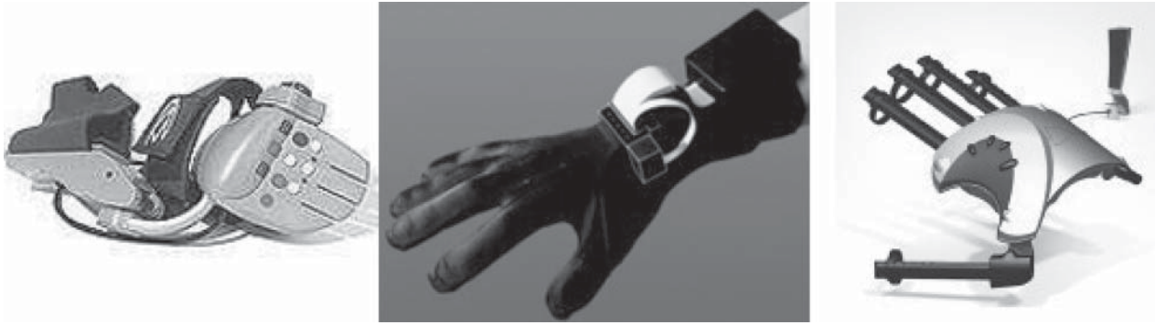
Figure 5. Three of the many glove controllers in use: Reality Quest N64 NGlove (left), P5 3D Virtual Glove (centre), and the 5DT Data Glove (right).
