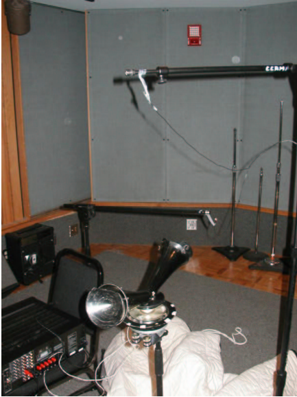
Figure 4: Rotating horn recording set up.
