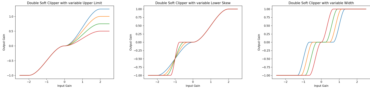
Figure 6: Double soft clippers with variable upper clipping limit (left), variable lower skew (middle), and variable dropout width (right).
