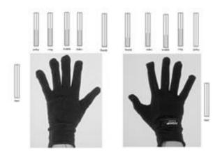
Figure 6: A Max (MSP) patch is used to demonstrate the sensitivity and resolution of the sensors. Each finger and heel of the glove is mapped to a level meter, and gives visual feedback to the amount of pressure being applied.
