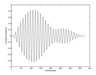
Figure 5: The waveform from figure 4 after being passed through a Helmholtz resonator representing the cicada's abdominal air sac.
