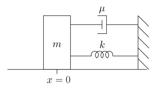
We will use such ODEs to model mass, spring, and dashpot elements, and their equivalent circuits
