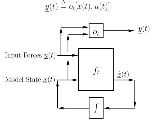
Usually the output is a *linear combination* of state variables and possibly the current input:
