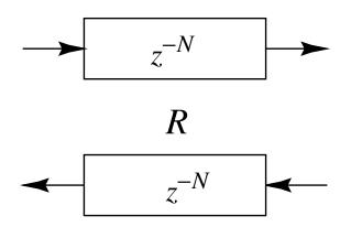
A digital waveguide is defined as a bidirectional delay line at some wave impedance  ${\cal R}$
