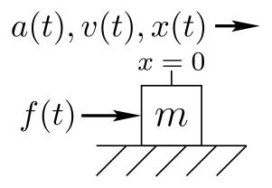
Force f(t) driving mass m along frictionless surface
