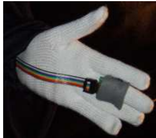
Figure 1: Accelerometer attached to hand
