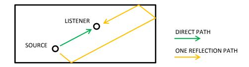
Artificial reverberation represents a very challenging problem, presenting a very **high computational cost** when modeled **from** a purely **physical perspective** (too many computations needed to simulate sound propagation in a 3D space).
