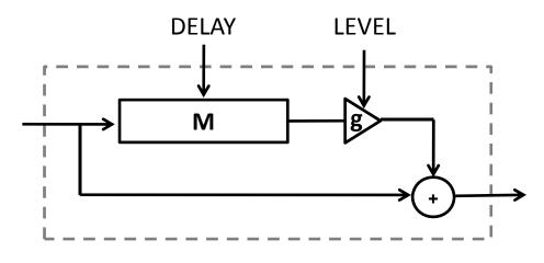
If the 'DELAY' control is set to be expressed in 'seconds', such value will have to be converted to 'number of samples'...
