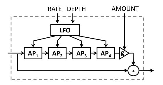
**Notches** in magnitude response **are finite** (as a function of the number of stages.
