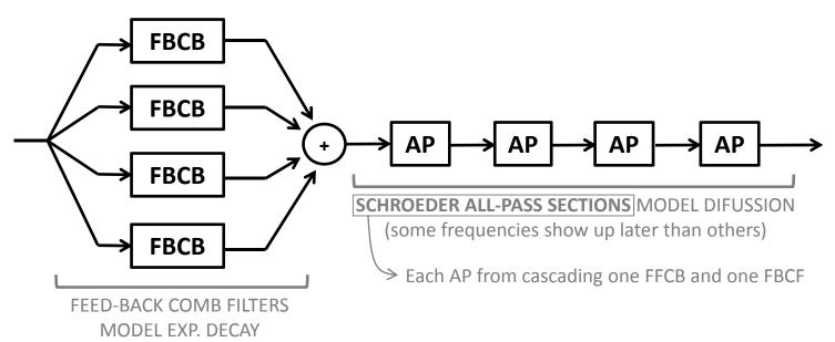
Delay line lengths must be set to be **mutually prime**, so **pd** 'Freeverb' smooth decay and echo density increase are ensured.
