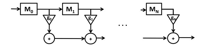
It is suggested that none of the taps' delay exceeds **40-50ms**, since it is acknowledged as the threshold for echo perception.
