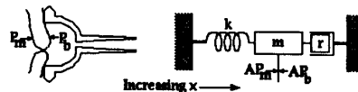
Figure 1: A drawing of the lips as placed on the mouthpiece, and a simplified physical model of the upper lip.
