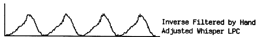
Figure 1.23: Waveform of normal mode phonation of the vowel /i/, after inverse filtering by hand adjusted whispered speech LPC filter.
