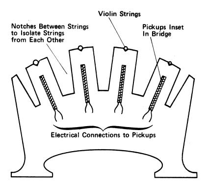
Figure 2. Sketch of Violin Bridge with Bimorphic Pickups
