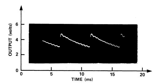
Figure 3. Output of Bender Pickup Mounted in Cello Bridge
