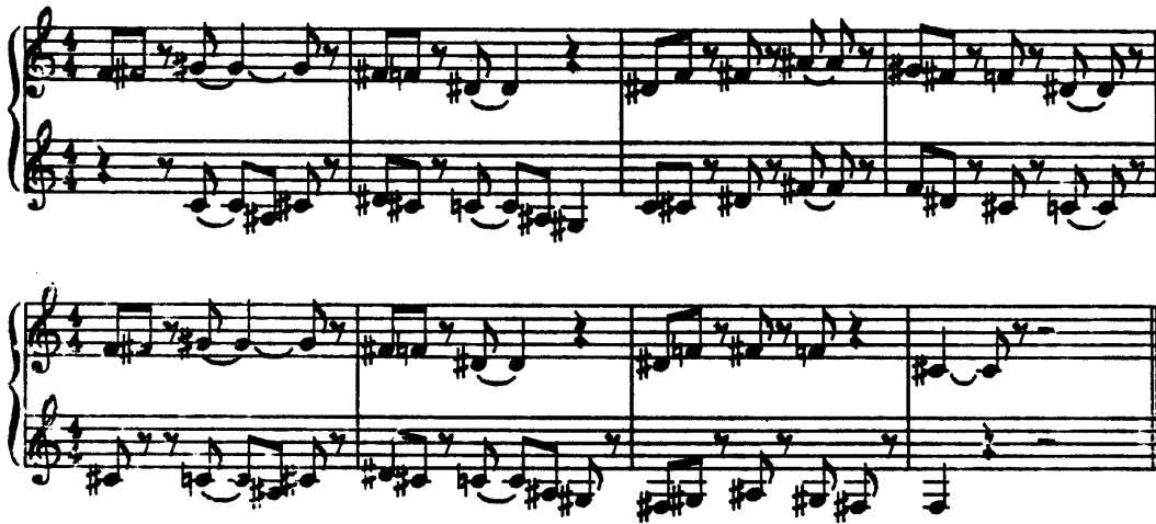
FIGURE 61. This is the score produced by the computer. Again, the lengths of the longer notes are consistently underestimated. Also, there is a note missing in the last measure. The most conspicuous change, however, is due to the fact that the guitar was mistuned somewhat high. The literal-minded computer faithfully reports the score here one half-step high throughout. The intervals between consecutive notes is correct in terms of the number of half-steps the interval represents. Please note that this is not good musical notational style. This should be notated in the key of Db, which would make all the accidentals disappear. We retain this notation because it is simple, general, and can represent 12-tone pieces as well as tonal pieces, although the representation is quite clumsy in many cases.
