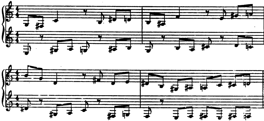
FIGURE 59. This is the score produced by the computer. The lengths of the longer notes are consistently underestimated. This is because the threshold for noise rejection is set so high that the tail ends of the notes are lost.
