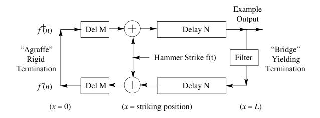
"Waveguide Canonical Form"
