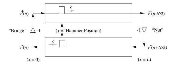
Initial conditions for the ideal struck string in a *velocity* wave simulation.
