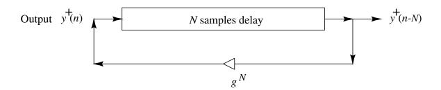
All N loss factors g have been "pushed" through delay elements and combined at a *single* point.
