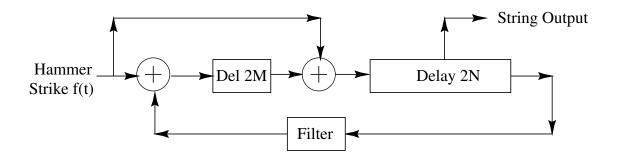
Finally, we "pull out" the comb-filter component:
