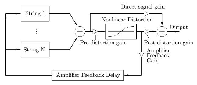
Distorted Electric Guitar with Amplifier Feedback
